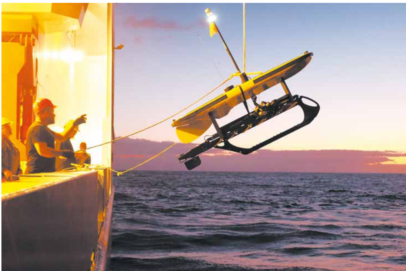
Deployment of a wave glider from RV SONNE offshore Northern Chile during a seafloor geodesy experiment for absolute positioning.
