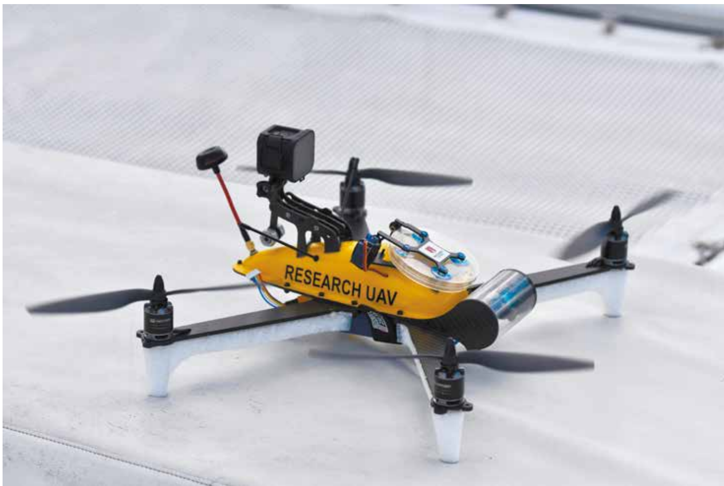
Purpose-built UAV designed to sample whale blow. Pirotta et al., 2017.
