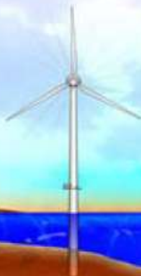
Monopile Foundation depth 0 – 30 m
