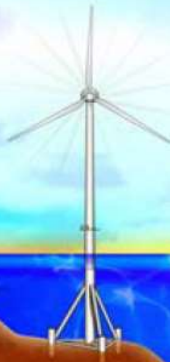
Tripod fixed bottom depth 20 - 80 m
