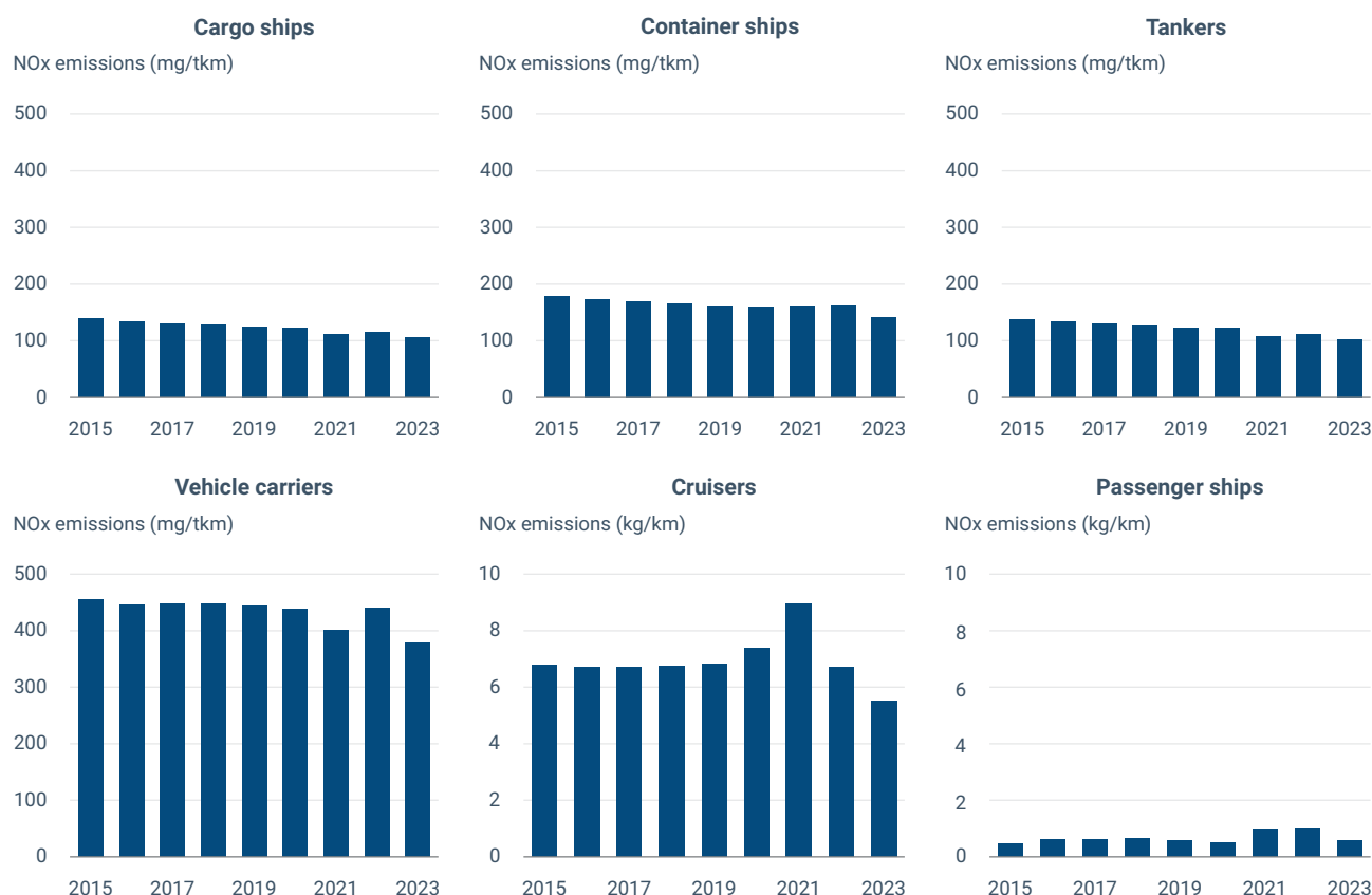
Figure 2.13 NOx specific emissions from selected freight and passenger ship types in the EU-27
